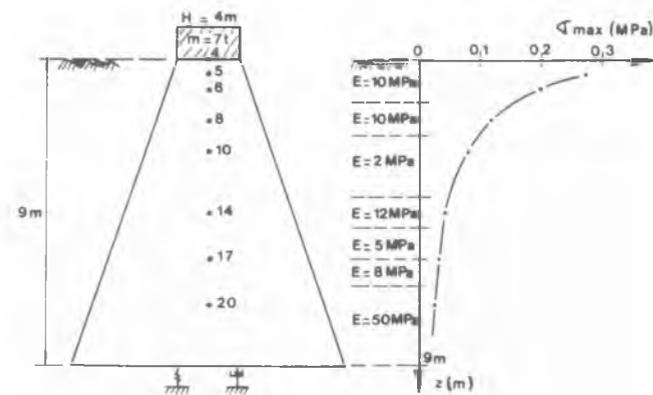
Figure 4 a) Model b) Dynamic stress vs. depth
