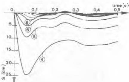
Figure 5 b) Displacements at various depths
