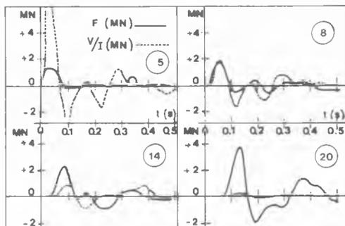
Figure 5 a) Force and velocity at various depths
