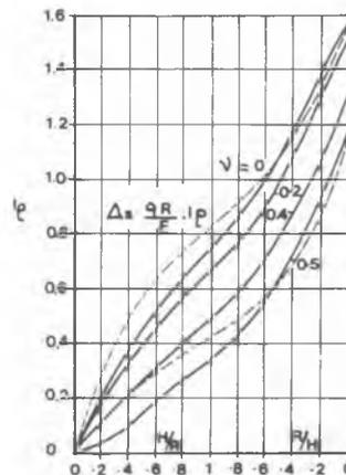
Figure 3 : Deflection on finite elastic layer.
