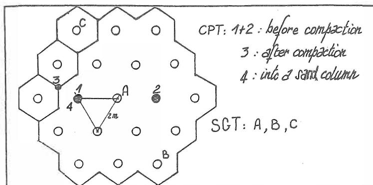
Fig. 1.a. Grid pattern of stone columns
