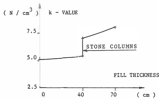
Fig. 9. Effect of reinforcement on measured k-value.
