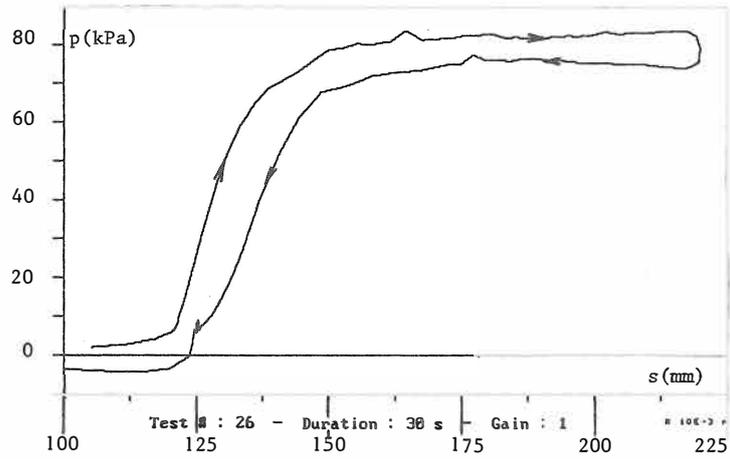
Fig. 3. Stress-displacement curve (1 kPa = 0.145 psi, 1 mm = 0.0394 in)
