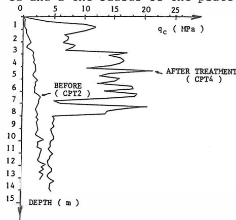
Fig. 10 CPT profiles before and in stone column, after treatment. (1 m = 3.28 and 1MPa = 6890 psi)
