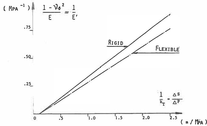
Fig. 7. Chart for direct interpretation of field tests.
