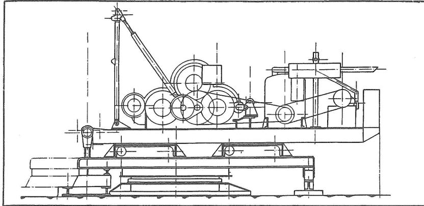
Fig. 2.a Sketch of walking mechanism of the piling rig.
