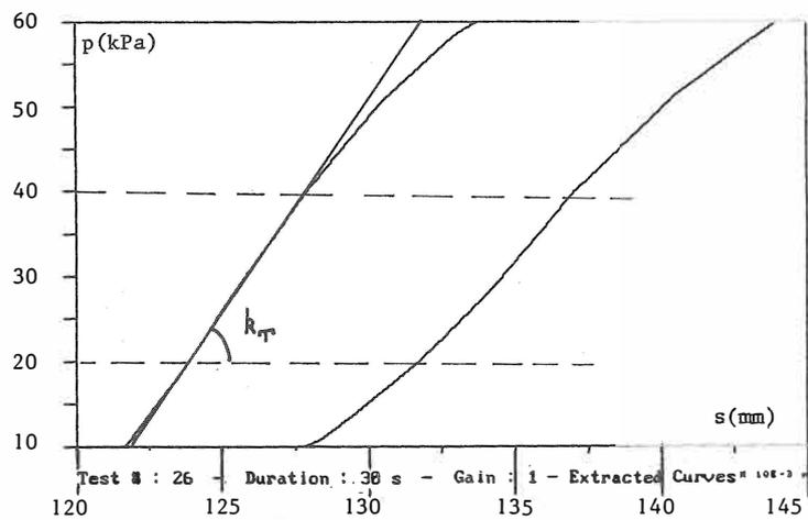
Fig. 4. Enlarged section of the load-deformation curve for detailed data interpretation (1 kPa = 0.145 psi, 1 mm = 0.0394 in)
