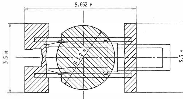
Fig. 6. Geometry of the central plate and outer beams.
