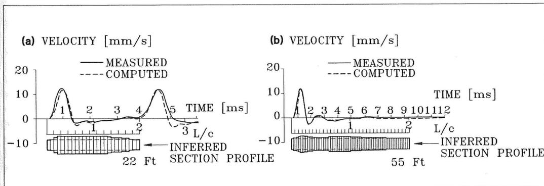
Fig. 5 - Pile Shape Evaluated from Signal Matching
