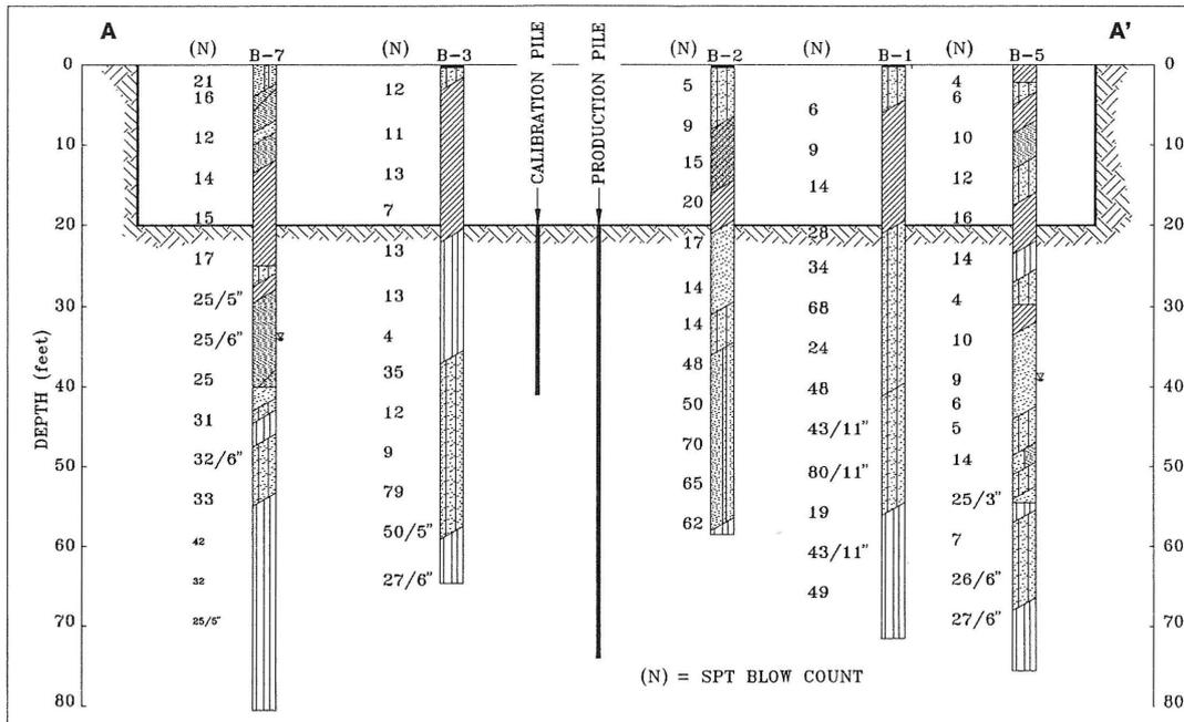
Fig. 2 - Geotechnical Cross-Section
