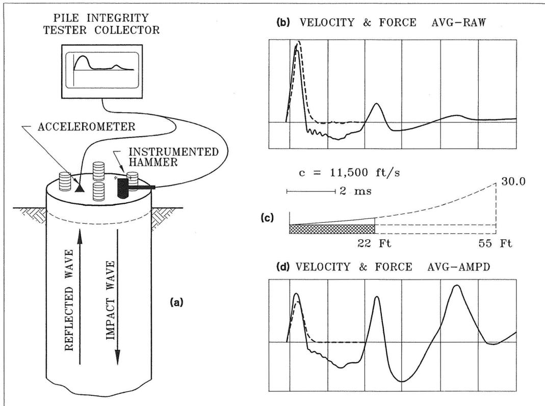
Fig. 3 - Integrity Testing Setup and Procedure
