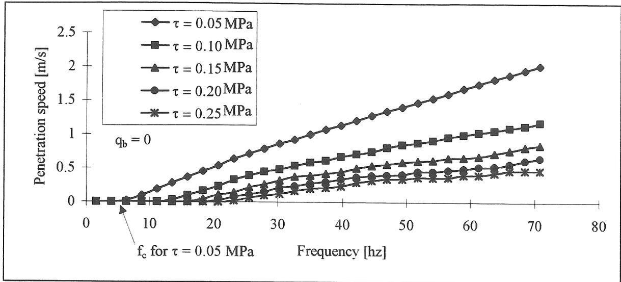
Figure 6: Evolution of the penetration speed in function of the frequency.
