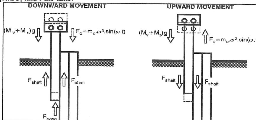
Figure 1: The different strengths applied to the sheet-pile.
