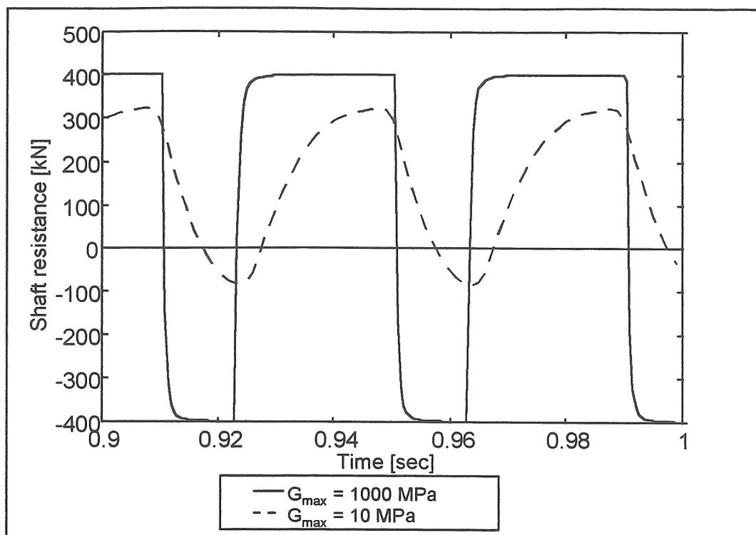
Figure 13: Comparison of shaft resistance for two shear modulus.
