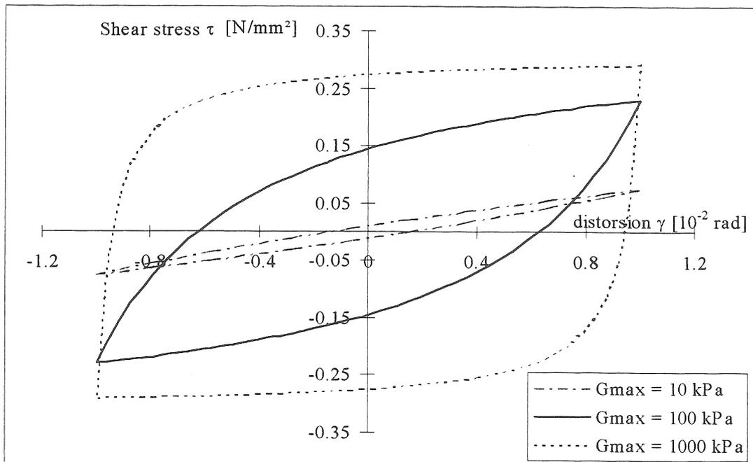
Figure 9: Stress-strain relationship during a cyclic deformation.
