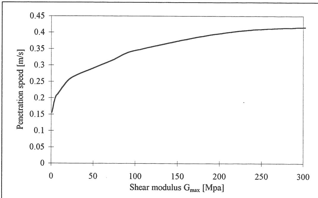
Figure 12: Evolution of the penetration speed in function of the shear modulus.
