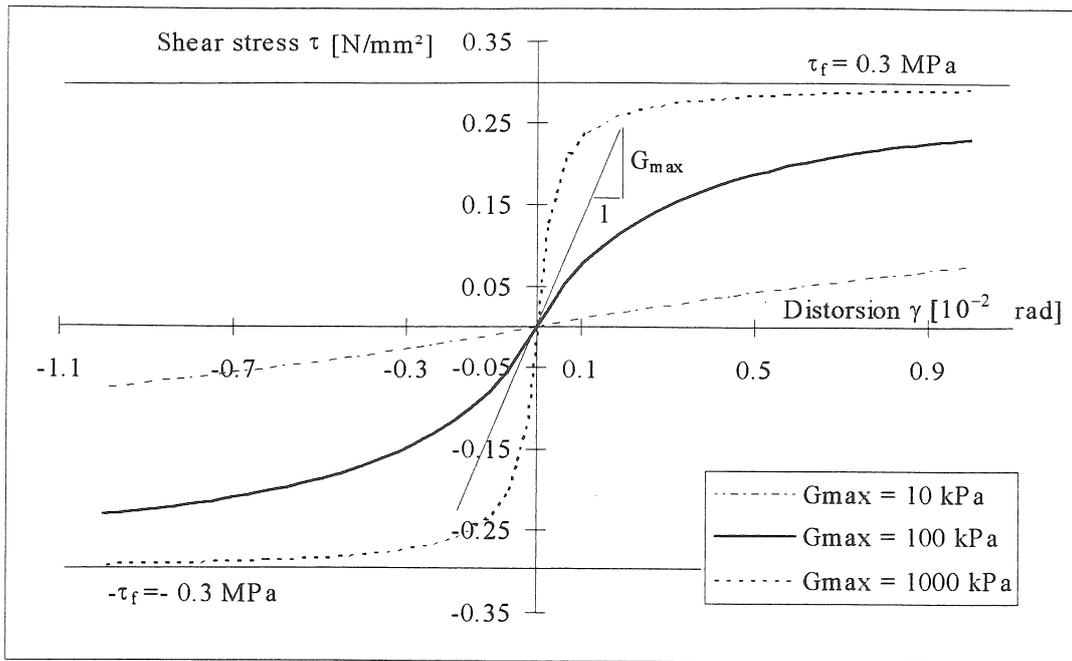
Figure 8: Static stress-strain relationship (hyperbolic model)
