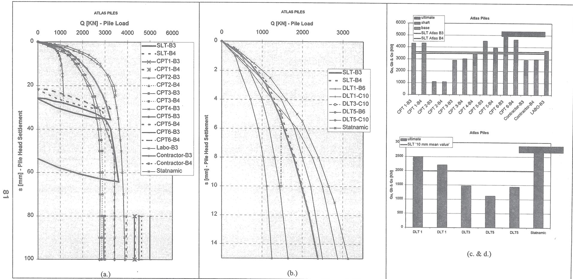
Figure 13 : Atlas pile results : a. & c. Static Prediction Load-settlement curves and Load Histogram
