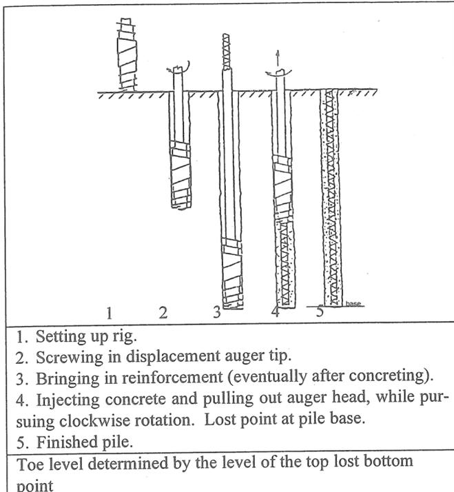
Figure 5. - Installation process of Omega Pile
