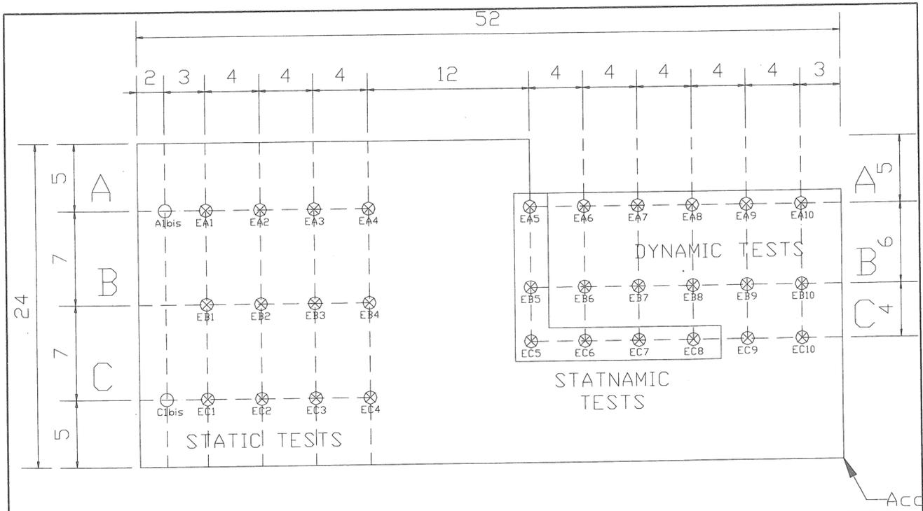
Figure 6 : Tests Piles Layout
