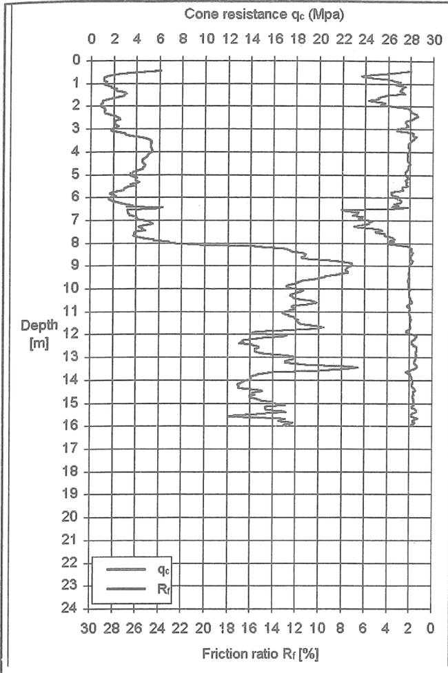
Figure 8 : CPT-E Result : cone resistance [Mpa] and Friction Ratio [%]
