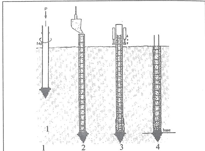
1. Screwing in tube, closed at the bottom with displacement auger tip.
