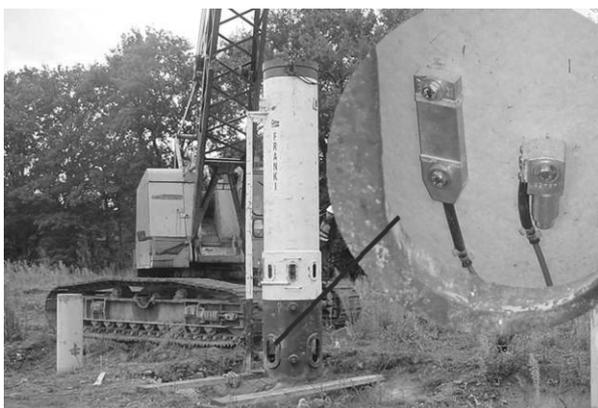
Fig 1: Hammer, pile and transducers details of a Dynamic Load Test
