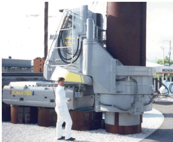
Figure 2. A 'press-in' piling machine for installing large tubular piles
