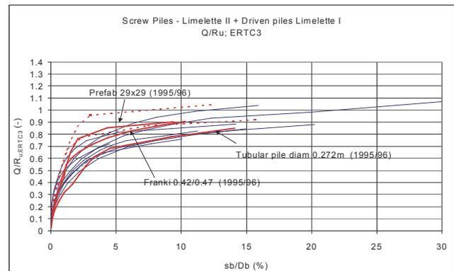
Figure 7. Normalised load settlement curves static pile load tests Limelette including results of an earlier test campaign (1995-1996) on driven displacement piles.
