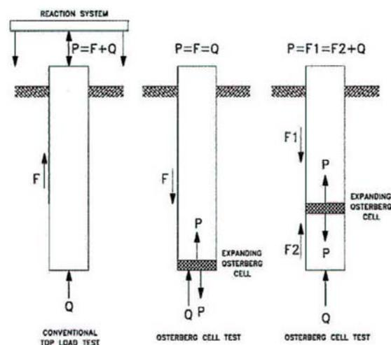
Fig. 5 – Comparison of Static Load tests (England, 2006)
