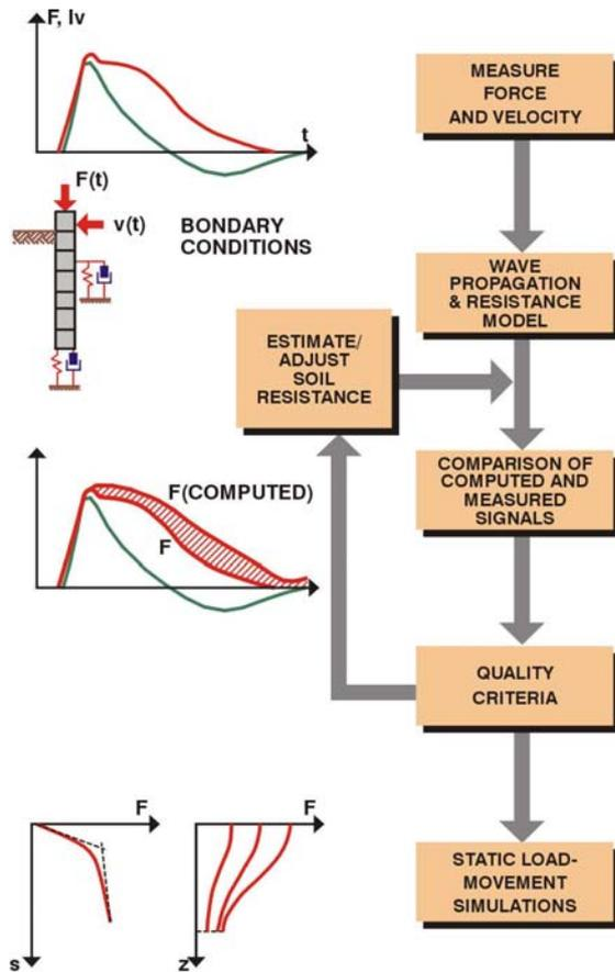
Fig. 15 – High-strain Inverse modeling to assess static load-settlement curve
