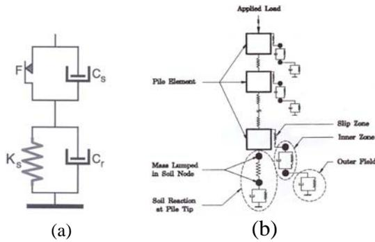
Fig. 19 - Soil-Pile dynamic interaction Models (a) Randolph & Deeks, 1992, (b) El Naggar & Novak, 1994
