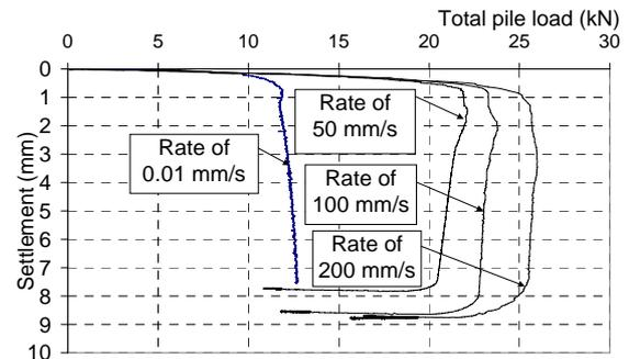
Fig. 20 – Model Pile Load-settlement curves at different penetration rates (*Anderson et al, 2006*)
