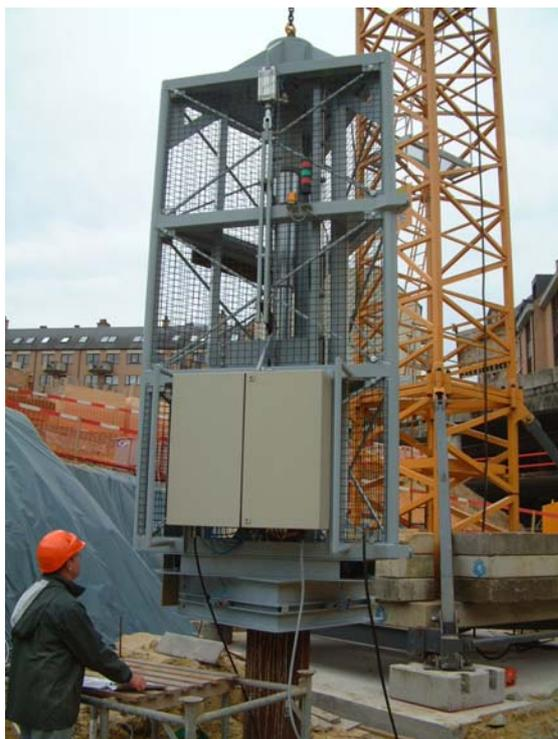
Fig. 13 – FonDyTest loading device
