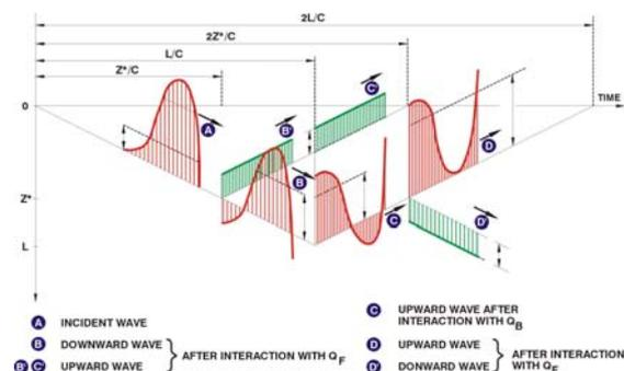
Fig. 14 – Wave generation and reflections in dynamically loaded pile.
