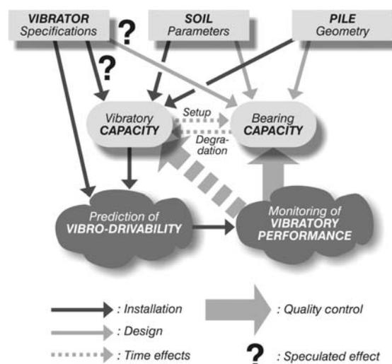
Fig. 2 – Monitoring of vibratory penetration (Holeyman et al, 2002)
