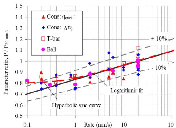
Fig. 22 – Effect of penetration rate on undrained resistance (*Randolph, 2004*)
