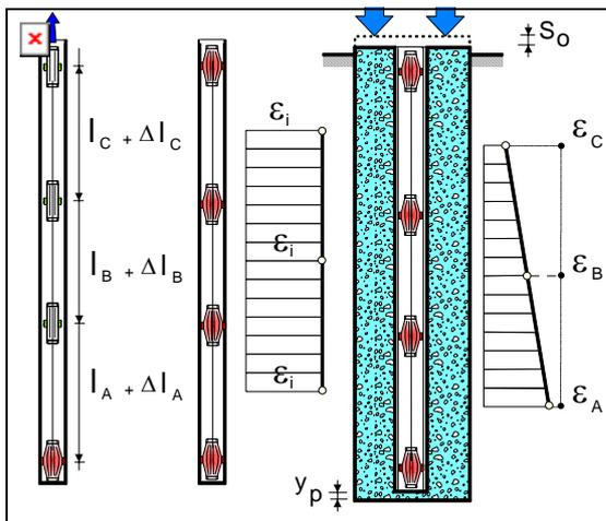
Fig. 7 – LCPC Extensometer Principle
