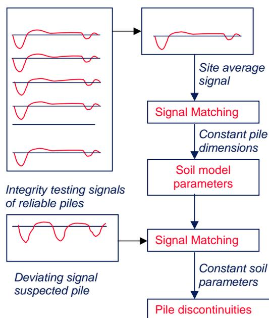
Fig. 24 – integrity testing signal matching procedure (*Middendorp et al., 2006*)
