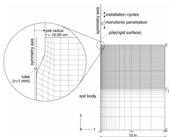
Fig. 25 – Finite Element Modelling of Pile Installation Process (*König & Grabe, 2006*)
