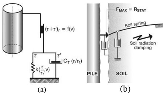
Fig. 18 – Simplified soil-Pile dynamic interaction Models (a) Holeyman, 1984, (b) Paquet, 1988
