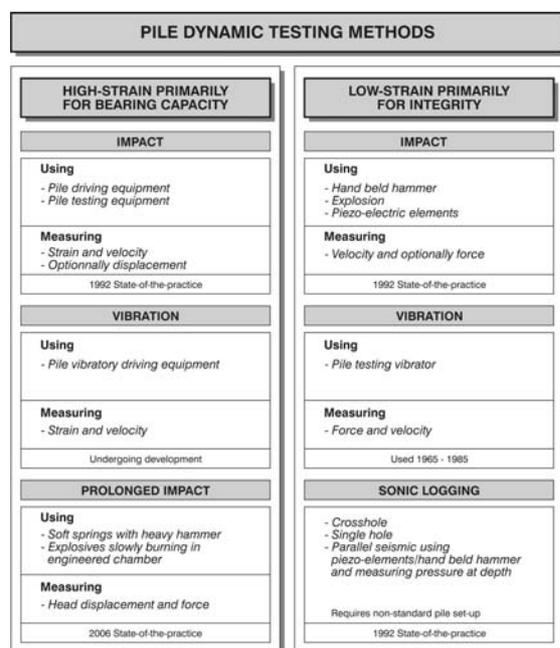
Fig. 3 – Pile dynamic testing methods
