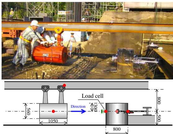
Fig. 12 – Manually actuated dynamic horizontal load test (Kojima *et al.*, 2006)
