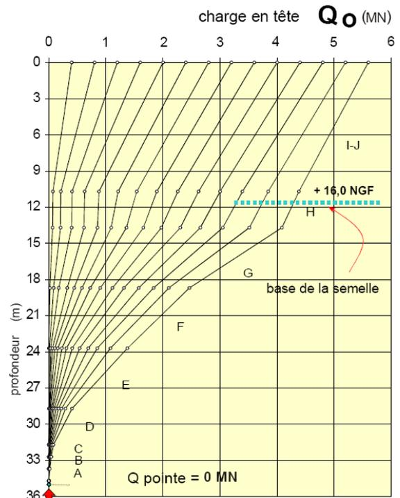
Fig. 8 – Typical results from LCPC extensometer instrumented pile test (Bustamante, 2005)
