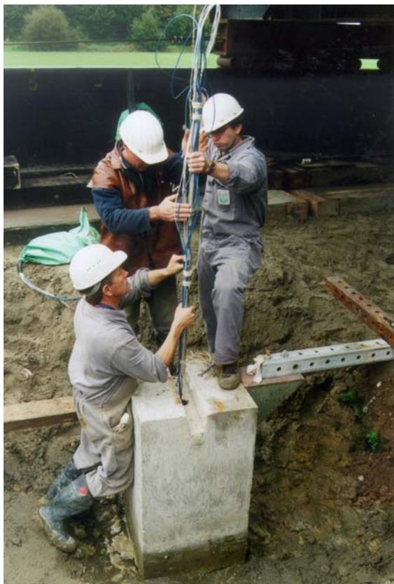
Fig.9 – Insertion of segmental extensometers in test pile (Huybrechts, 2001)
