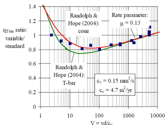
Fig. 23 - Penetration resistance from T-bar "twitch" tests (Randolph, 2005)
