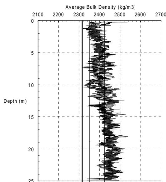
Fig. 10 - Gamma-gamma density profiles from 5 access tubes within 1.5 m diameter bored pile (Courtesy of EarthSpectives, 2006)
