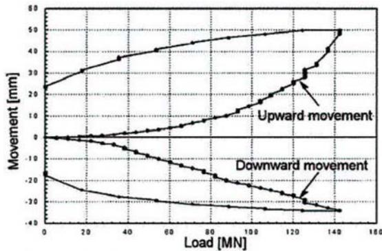
Fig. 6 - High Capacity Load-Movement Curves (England, 2006)
