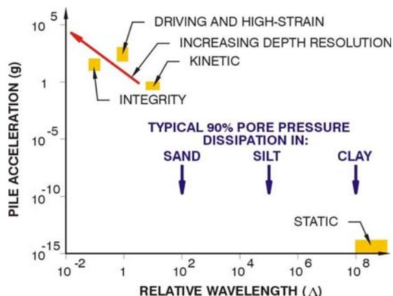
Fig. 4 – Sharpness and duration of force pulse for different pile tests
