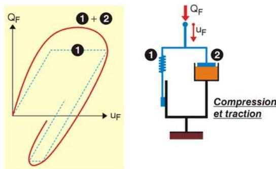
Fig. 16 – Basic form of damping (of the Smith, 1960)
