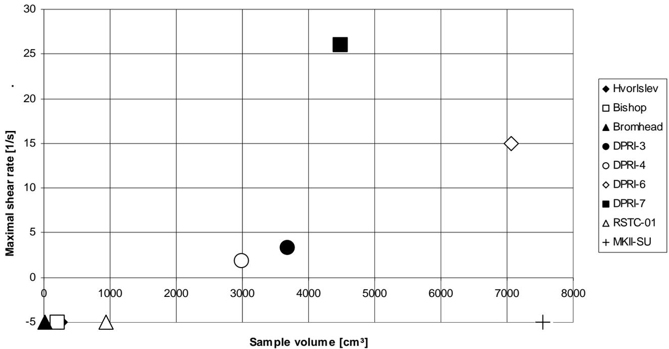
Figure 10. Comparison of ring shear testers – sample volume and shear rate (based on the values from table I)
