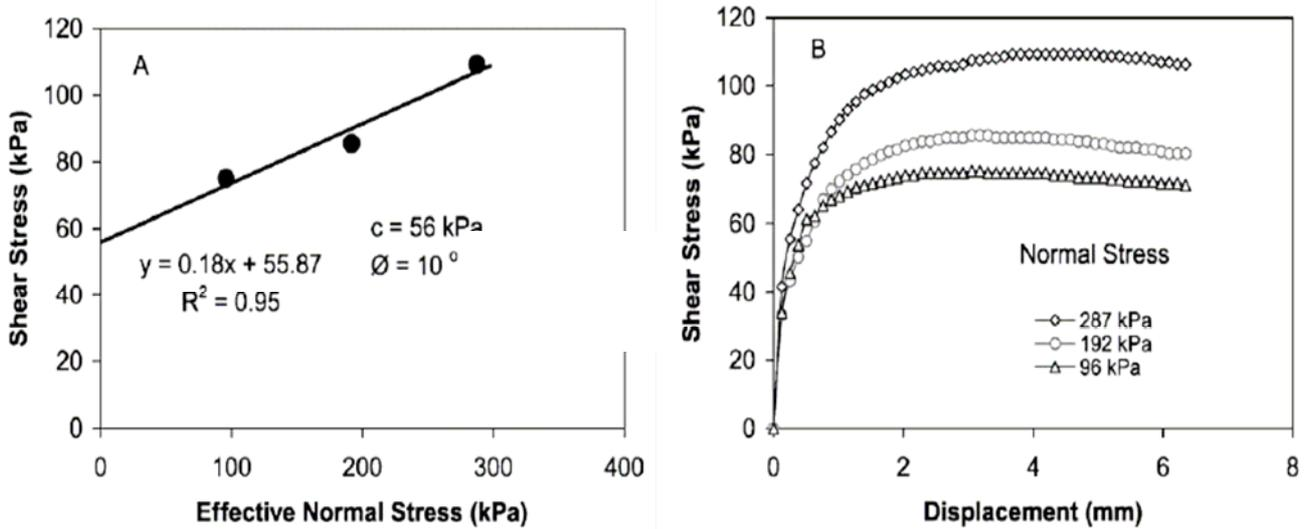
Figure 11. Example of result curves of ring shear tests (from Wan & Kwong 2002)
