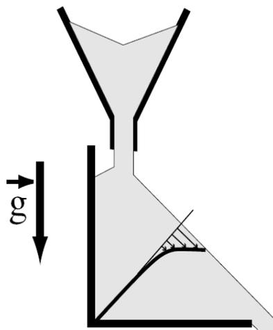
Figure 6. Heap flow (from GDR MiDi 2004)
