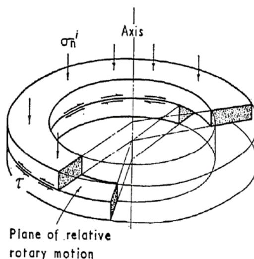
Figure 4. Ring shear testing geometry (from Bishop et al. 1971)
