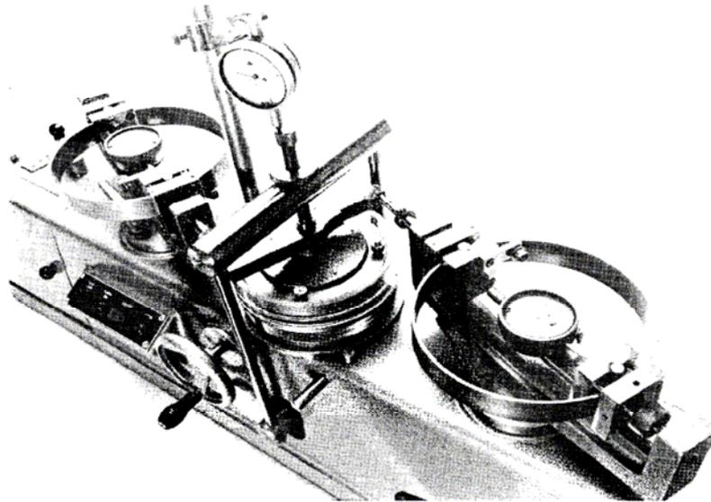
Figure 9. Bromhead ring shear tester, commercial version (from Bromhead 1979)
