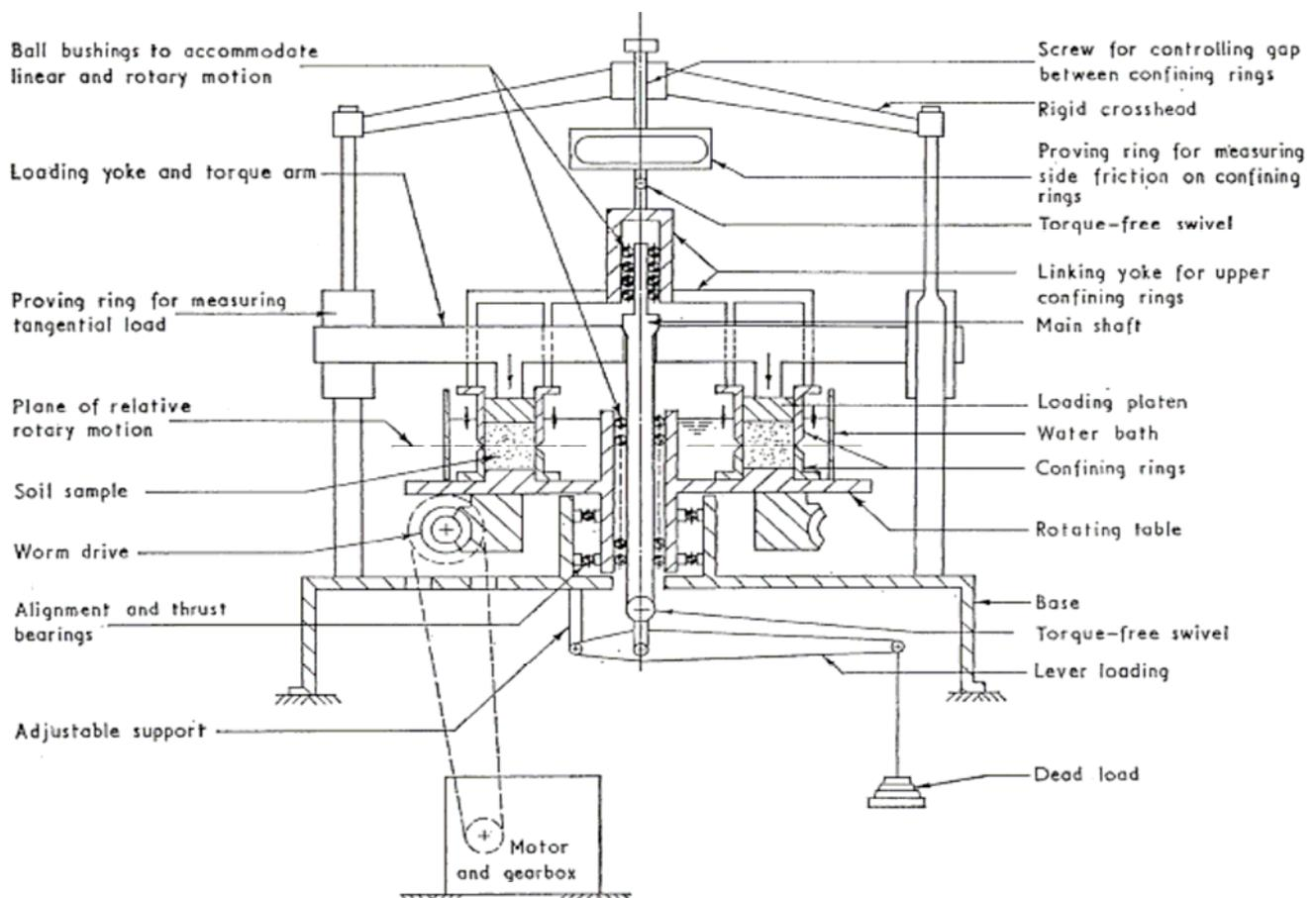
Figure 8. Bishop ring shear tester (simplified section, from Bishop et al. 1971)
