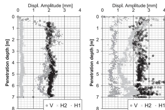
Figure 10. Lateral movements of sheet piles vibro-driven at the Limelette test site, (a) with one clamp positioned on the flange of the sheet pile, (b) with two clamps positioned on the webs of the sheet pile – Sheet pile no 2, Limelette (2007).
