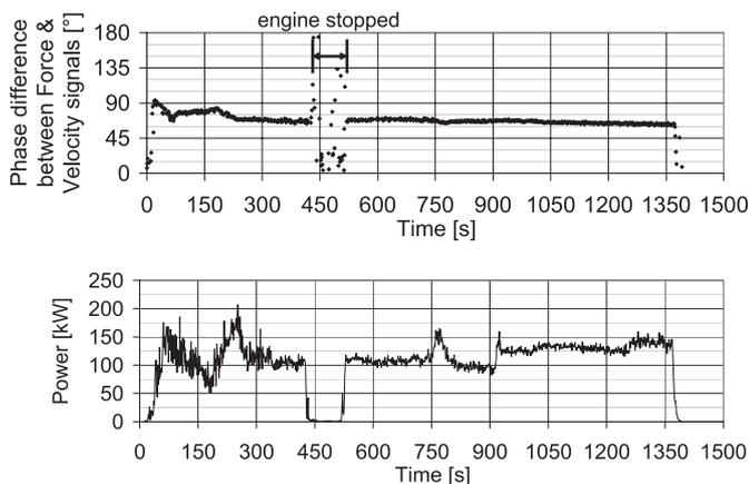
Figure 6. Phase difference between velocity and force & calculated transmitted power – sheet pile no 1, Limelette (2004).
