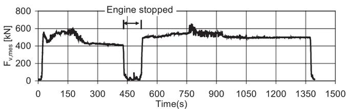
Figure 5. Measured vibratory part of the driving force – Limelette 2004.
