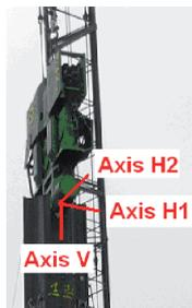
Figure 9. Definition of axes H1, H2 and V.
