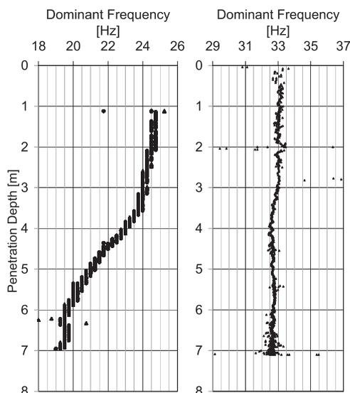
Figure 3. Evolution of the dominant frequency in function of the penetration depth: (a) Sheet pile tested at Merville, (b) Sheet pile no 1 tested at Limelette 2004.
