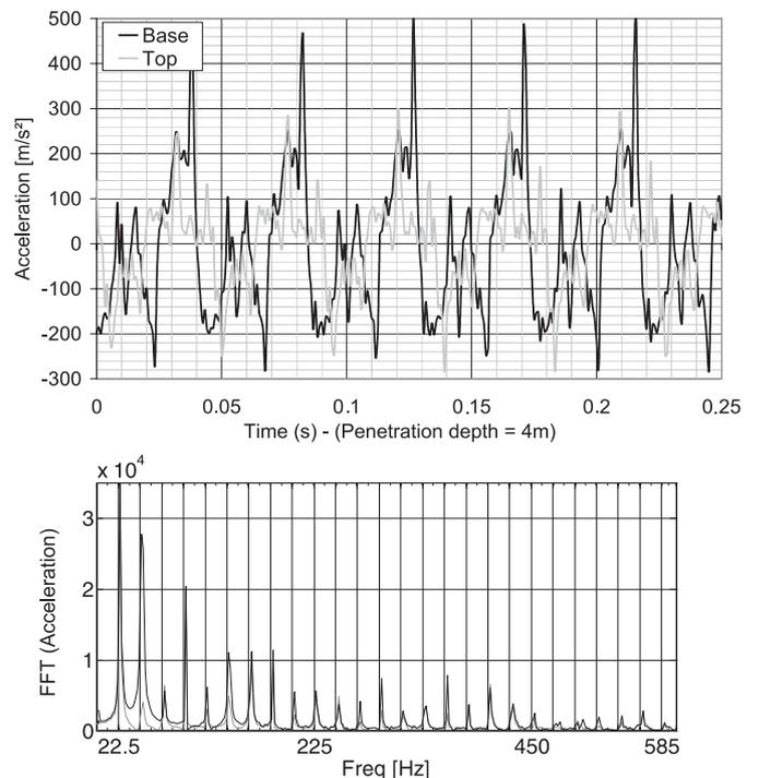
Figure 11. Detail of an acceleration signal obtained at Montoir – (a) time record, (b) frequency analysis.
