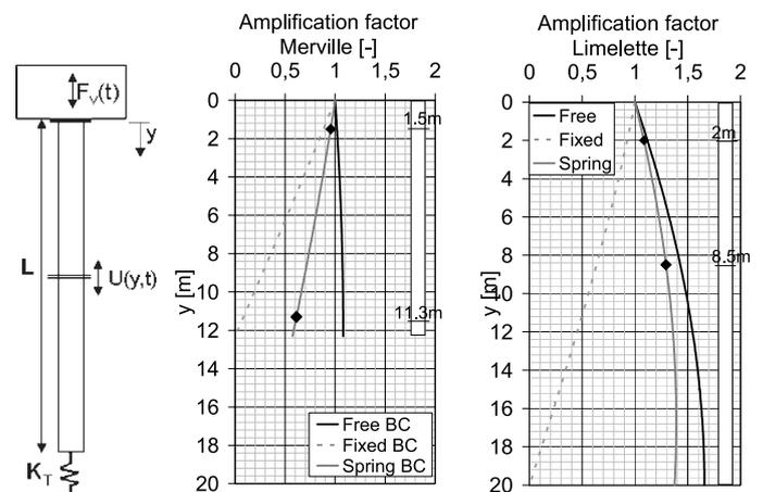
Figure 8. Amplification factors of the displacement amplitudes, deduced from the steady state solutions and expressed as a function of the position of measurement on the profile.
