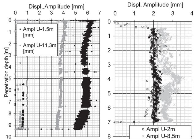
Figure 7. Displacement amplitude for (a) the tube tested at Merville (position of the measurements: 1.5 m and 11.3 m from the top), (b) the sheet pile no 2 tested at Limelette (2007) (position of the measurements: 2 m and 8.5 m from the top).
