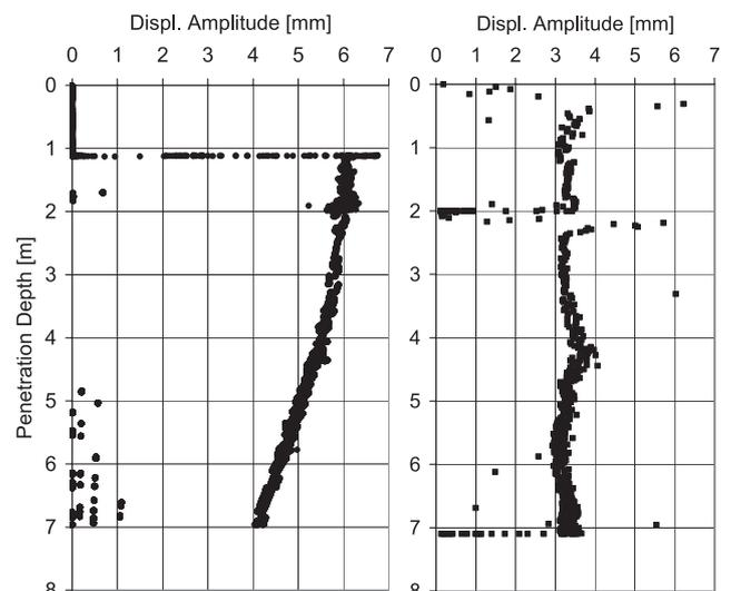
Figure 4. Evolution of the vibratory amplitude in function of the penetration depth: (a) Top of sheet pile tested at Merville, (b) Top of sheet pile no 1 tested at Limelette 2004.
