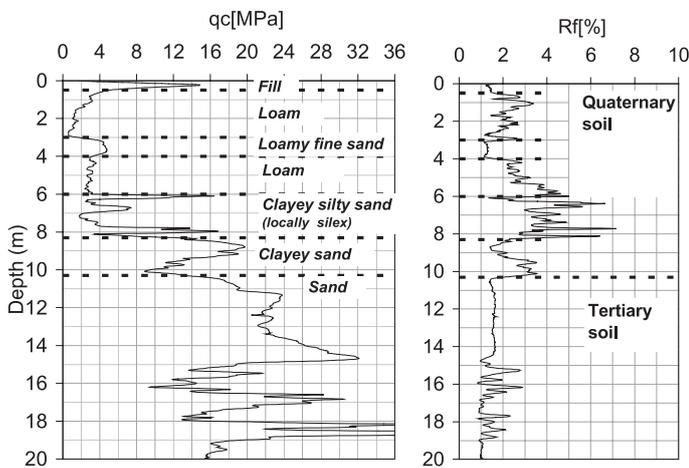
Figure 2. CPT-E results – Test site of Limelette.
