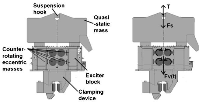
Figure 1. Example of vibrator (ICE 36RF-ts).
