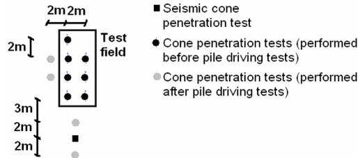
Figure 1. Implantation of the CPTs and sheet pile driving tests
