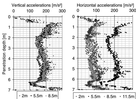
Figure 7. Vertical & horizontal acceleration amplitudes of the sheet pile measured at 2m, 5.5m and 8.5m from top of the sheet pile (Hd test)
