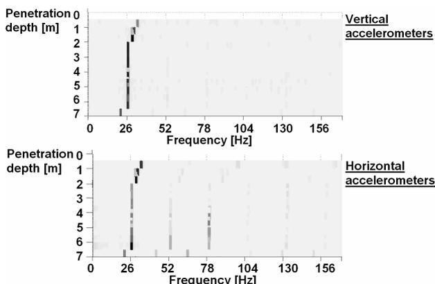
Figure 6. Spectral analysis of vertical & horizontal sheet pile accelerations at 2m, 5.5m & 8.5m from top of the sheet pile (Hd test)
