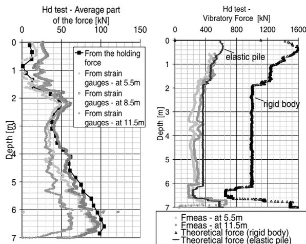
Figure 8. Strain gauges transducers results (measurements performed at 5.5m, 8.5m and 11.5m from the sheet pile top) as a function of the penetration depth
