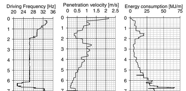
Figure 5. Driving frequency, penetration velocity and energy consumption for test Hd (as functions of the penetration depth)
