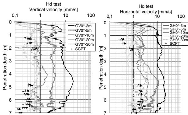
Figure 10. Soil particle velocities measured for test Hd. GV(H)-...m = Geophone measuring the vertical (horizontal) direction, at a distance of m from the sheet pile. The SCPT measurements have been performed at a distance of 9m from the pile, at a depth of 3.9m.
