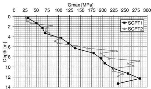
Figure 3. Small strain shear modulus deduced from seismic cone penetration tests results
