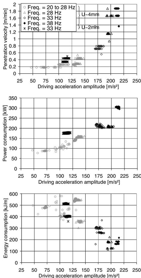
Figure 11. Penetration velocity, power and energy consumption obtained for the 11 driving tests as a function of the driving acceleration amplitude (for a pile penetration depth between 6 to 6.5m)
