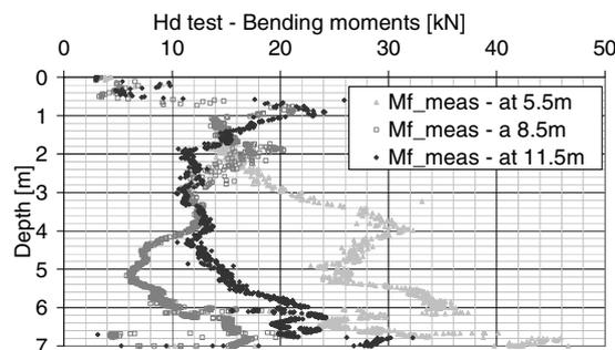
Figure 9. (Total) Bending moments deduced from strain gauges measurement performed at 5.5m, 8.5m and 11.5m from the sheet pile top (as a function of the penetration depth)
