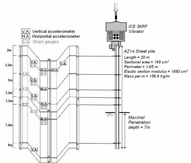
Figure 4. Position of the transducers on the sheet pile along with sheet pile and vibratory equipment
