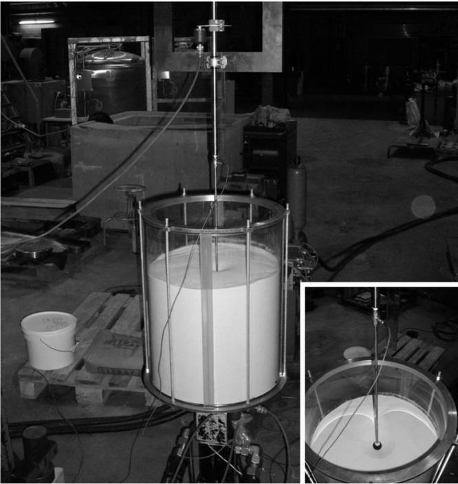
Fig. 10. UCL Sphere Penetration Experiment (SPE) apparatus, after Denies et al. (2009).
