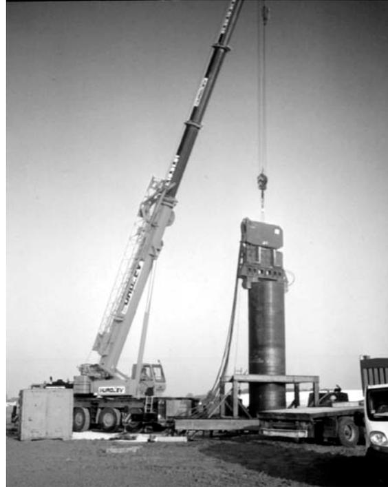
*Fig. 1. Steel pile driven with vibrator in Belleville (F) (<http://www.leductp.com/>).*
