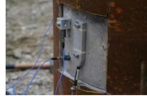
Figure 3: DLTM transported in field      Figure 4 : strain gauge and accelerometers on pile head
